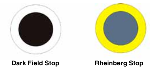
Figure 2. Examples of dark field and Rheinberg color stop.
