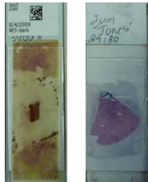
Figure 4. Examples of “mirroring”/grey haze. The cause of this effect is over-heating of the methenamine solution.
