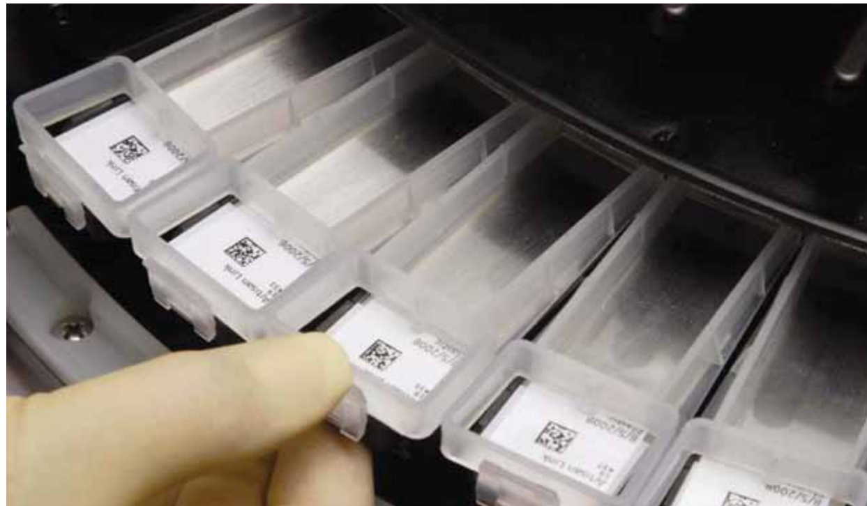
Figure 1. A. Early, breadboard-version slide chamber for containing staining reagents, with a slide inserted under one of the chambers. B. Line drawing of an individual slide chamber from the patent illustration, showing the spring-loaded mechanism for maintaining downward pressure. C. Picture of the current version of the slide clip, in the commercial version of the Artisan™.
